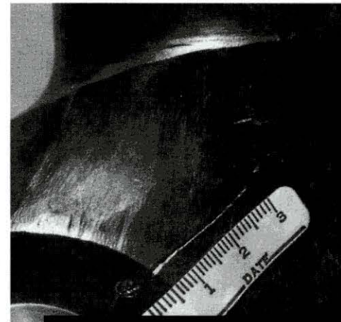
Figure 2 Crack in an older spray nozzle design.
